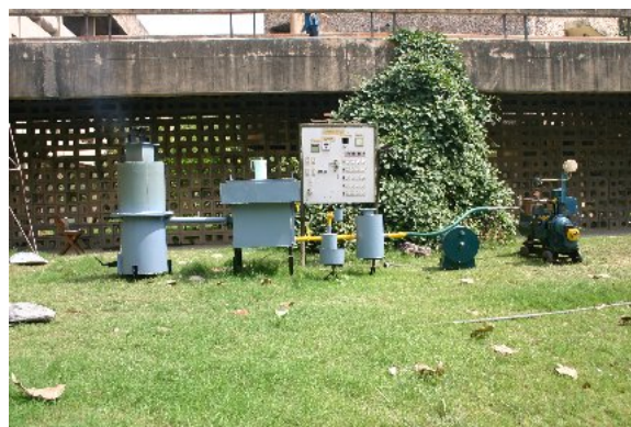
Figure 1: Gasifier engine system
